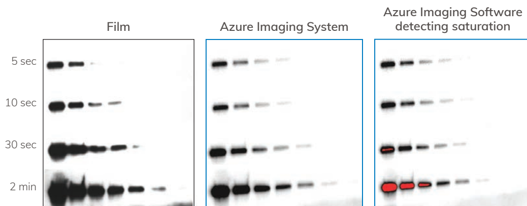
Figure 1. Saturation detection prevents errors in quantitation. The same blot was imaged on both x-ray film and the Azure Imaging System. The Azure system detects when CCD saturation occurs and calculates an auto-exposure time to avoid saturated bands.
